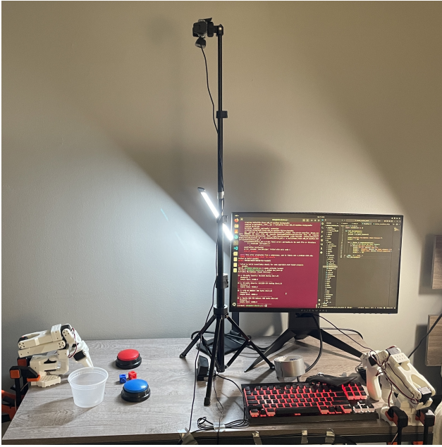
Figure 8. Data collection setup with SO-101 Leader arm pictured on the right, SO-101 Follower arm pictured on left, and cameras with microphone in middle.
